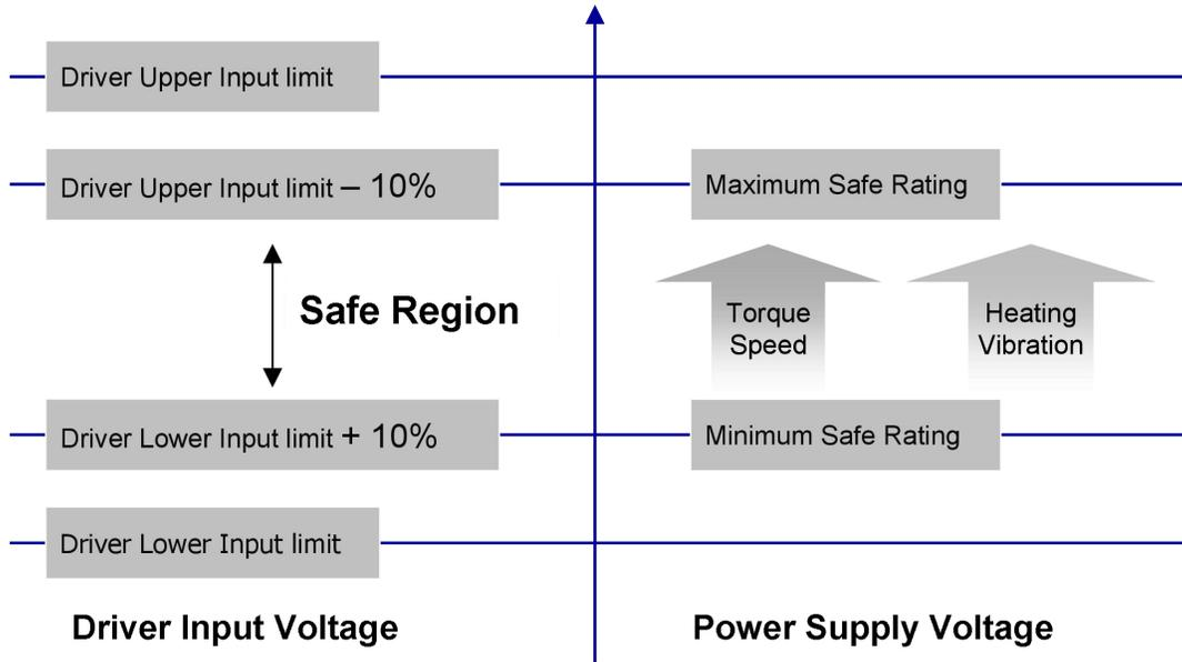
The recommended power supply voltage for DM805-AI is 24-72VDC:
