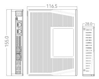
• Note: This is the dimension of 2CS3EIP series, also same to 2EM3EIP series.
