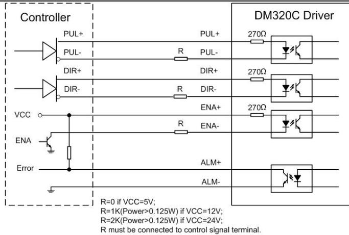
Figure 3: Connections to differential control signal
