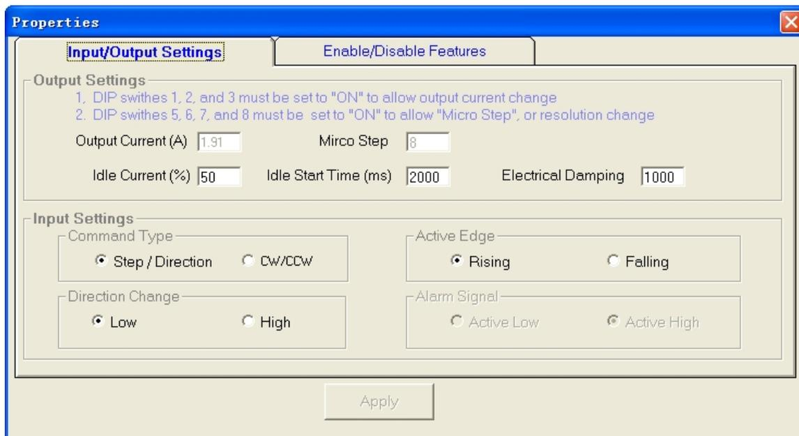
In most of the application, it is required to set only the output current, Micro Step and Command. Usually, the motor manufacturer states the RMS (root mean square) current in datasheet. Please refer to the hardware installation manual for how to set the output current.
