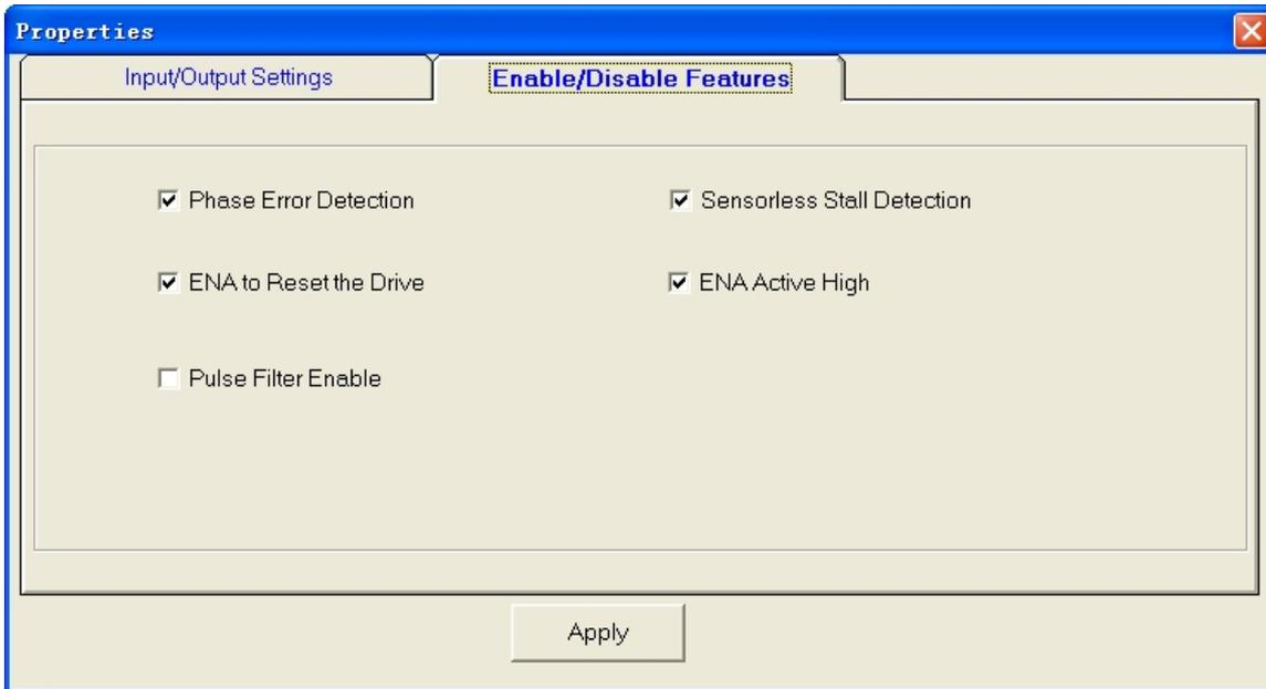
This window offers options of enabling phase error detection, motor stall detection and pulse filter. You can also set the active signal of the enable signal and use it for drive reset to clear the error.
