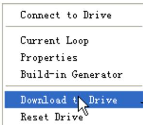
Save all the changes to the drive's non-volatile nonvolatile memory. You need to close the current tuning window firstly.
