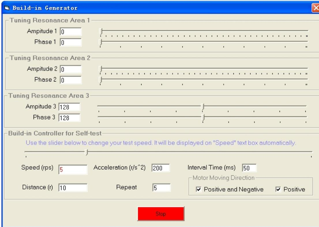
You can adjust the anti-resonance parameters in this window. The built-in controller can be used for anti-resonance tuning and self test.
