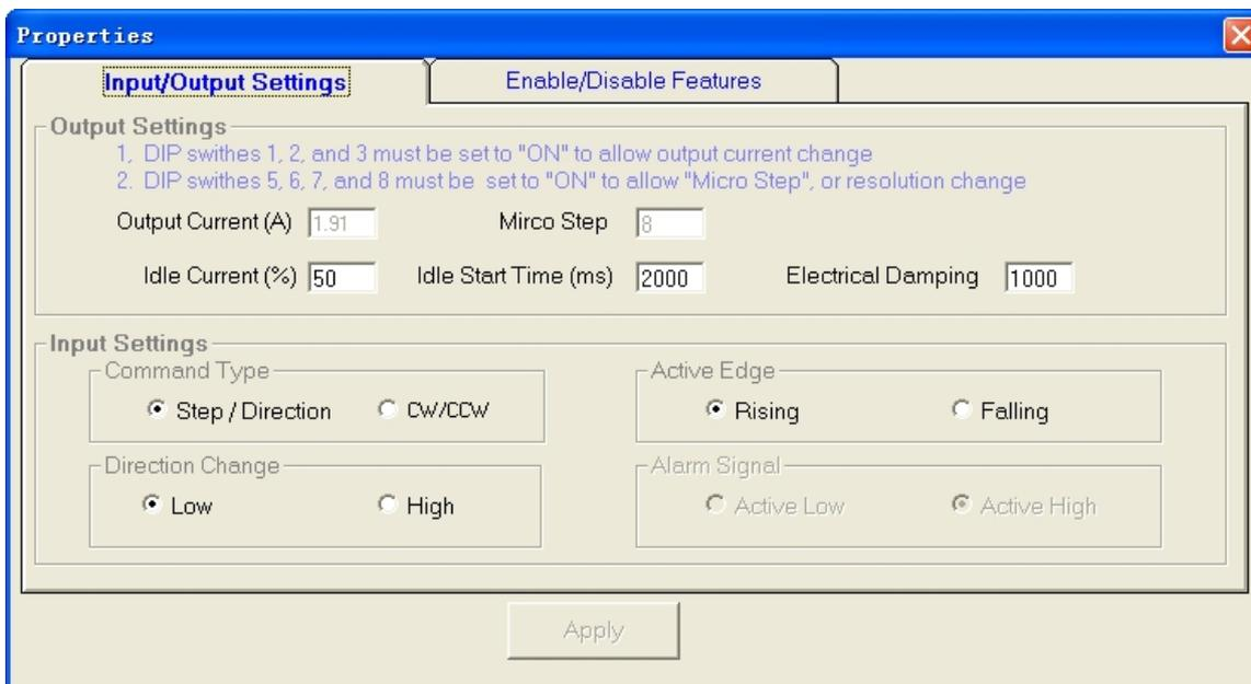
Click **Drive->Properties** to open the **Properties** window. In the **Input/Output Settings** Tab, the user can set Output Current, Micro Step, Idle Current, Electronic Damping, Pulse Active Edge and Command Type.
