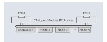
CANopen communication protocol with PDO settings for easier drive setup and 402 observer for drive data monitoring and tuning.
