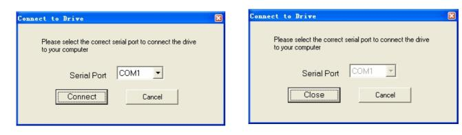
**Connect to Drive** window appears every time you open ProTuner. You can also open it by clicking **Connmunication>Connect To Drive** when the software is open. Select the serial port and click on the **Connect** button. The software will try to connect to the drive and read the settings. It may take several minutes. Please wait.
