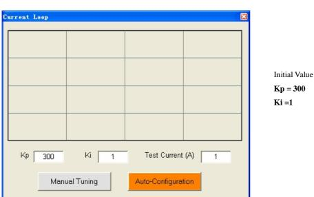
Step 1: Set Test Current 1 and start the tuning with small Kp and "zero" Ki. Here we set Kp=300 and Ki=1.
