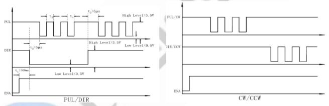
Figure 8: Sequence chart of control signals
