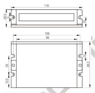
Figure 1: Mechanical specifications
