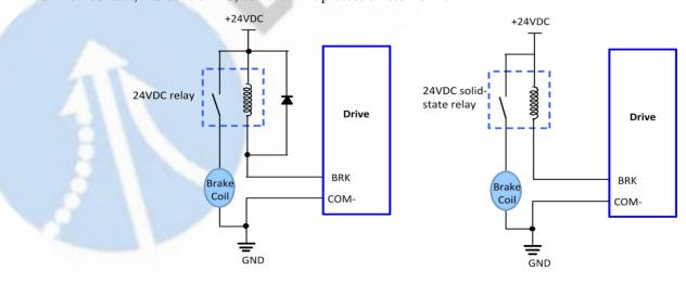
Figure 5: Brake Output Connection
