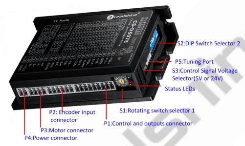
Figure 2: CS-D507E connectors
