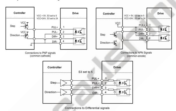
Figure 3: Control Signals Connection
