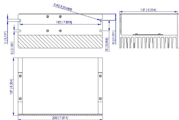
Figure 1: Mechanical specifications
